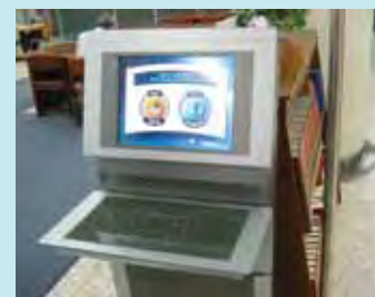
Readers place items they wish to refer to on the browse count RFID system before proceeding to the table to read them.
